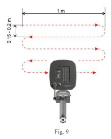
The antenna head should be held at a distance of 5-15 cm from the surface.
